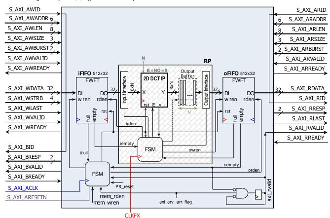
■ The input and output might require more than 32 bits. In this case, we need an input interface to the iFIFO and output interface to the oFIFO. The figure shows the different interfaces for each N (4, 8, 16) when B = NO = 8. The FSM @ CLK\_FX controls data flow from the input and the output, and as such, it depends on N.
